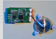
Thermoelectric harvester powering a wireless strain gauge
