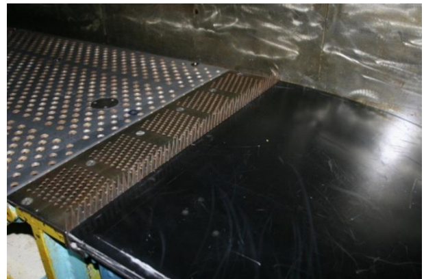
Fig. 2 - Spoilers at the entrance of the T-112 test section.
