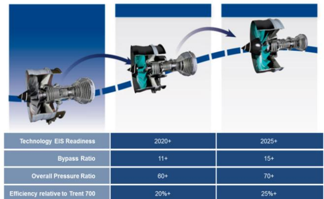
Figure 6: ADVANCE and UltraFan™ concept relative to Trent engine
