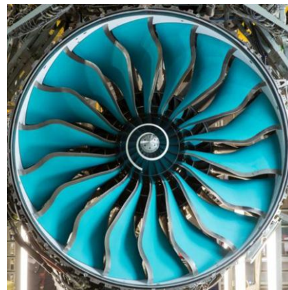
Figure 8: Composite CTi (Carbon/Titanium) Fan demonstrator ALPS (view from front).
