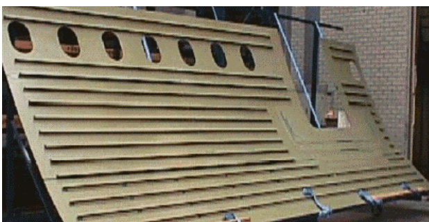
Fig. 4. GLARE ® shell with bonded stringers and doublers; A380 section 18, main deck panel
