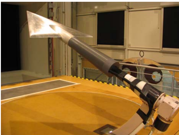
Fig. 3 Delta wing model mounted in test section of wind tunnel facility A.
