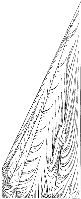
Fig.6 a. Surface streamlines of \alpha = 10.38^\circ using laminar boundary layer.
