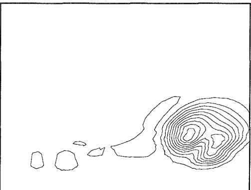
Fig.8 d. Total pressure contours at x/c_r = 1.05 for \alpha = 10.38^\circ using laminar boundary layer.
