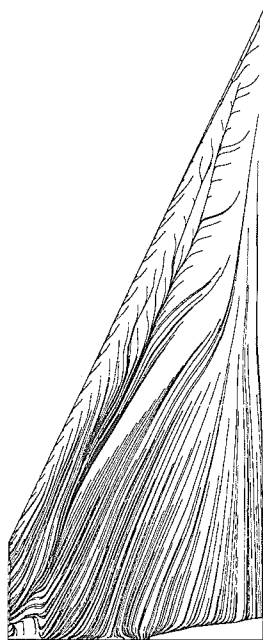
Fig.13 a. Surface streamlines of \alpha = 20.82^\circ using laminar boundary layer.
