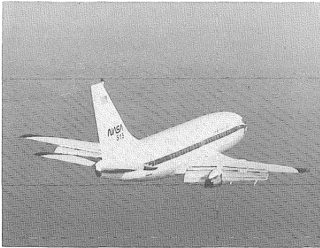
Figure 2. - NASA Langley TSRV (737-100 aircraft) in flight test of high-lift flap system aerodynamics.
