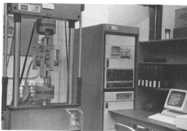
Fig. 10 View of Test Fixture and Beam Sample in MTS Fatigue Machine Providing FALSTAFF Spectrum Loading
