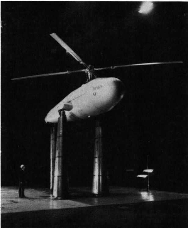
Figure 2. Full-scale rotor test apparatus in the Ames 40- By 80-Foot Wind Tunnel.
