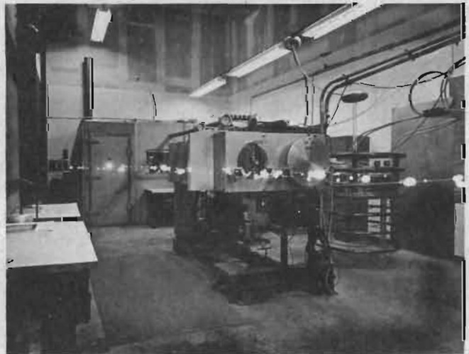
Figure 5. A practical realization of the E-beam sustainer laser. This laser produced 2,000 joules in 20 microseconds pulse with near diffraction limited performance. The hundred megawatt beam exploded dust particles in room air which produced the string of white beads in the photograph.
