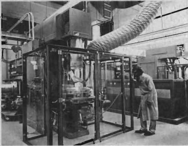
Figure 6. The Avco HPL-10 two station metal working laser. In this laser continuous operation at powers up to about 15 kW is achieved for industrial processing of metals. To facilitate more intensive use of the laser which is capable of operating continuously, two work stations are used so that set-ups can be made at one station while the other station is performing an operation. Lasers of this type have been sold to the Caterpillar Tractor Co. and the General Motors Corp.
