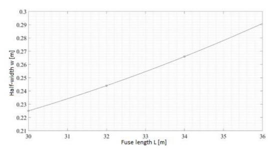
Figure 14 – Variation of optimal rib section width as a function of airship length.
