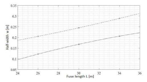
Figure 7 – Values of *L* and *w* guaranteeing vertical equilibrium solutions (continuous line), and structural limit solutions (dashed line) for an AI-Cu alloy rib.
