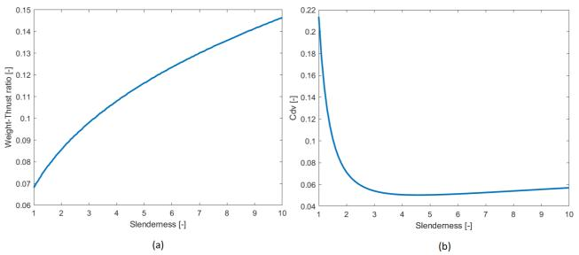
Figure 3 – Variation of (a) weight to thrust ratio, and (b) drag coefficient, as a function of slenderness.
