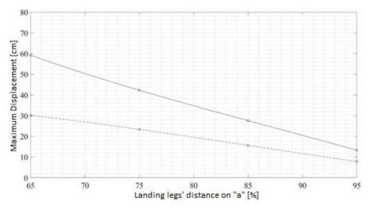
Figure 10- Variation of maximum displacement as a function of landing leg position for an AI-Cu alloy (continuous line), and composite (dotted line) rib.
