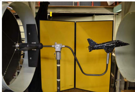
Figure 2 – Maneuver rig mounted in the open-jet section wind tunnel [5]
