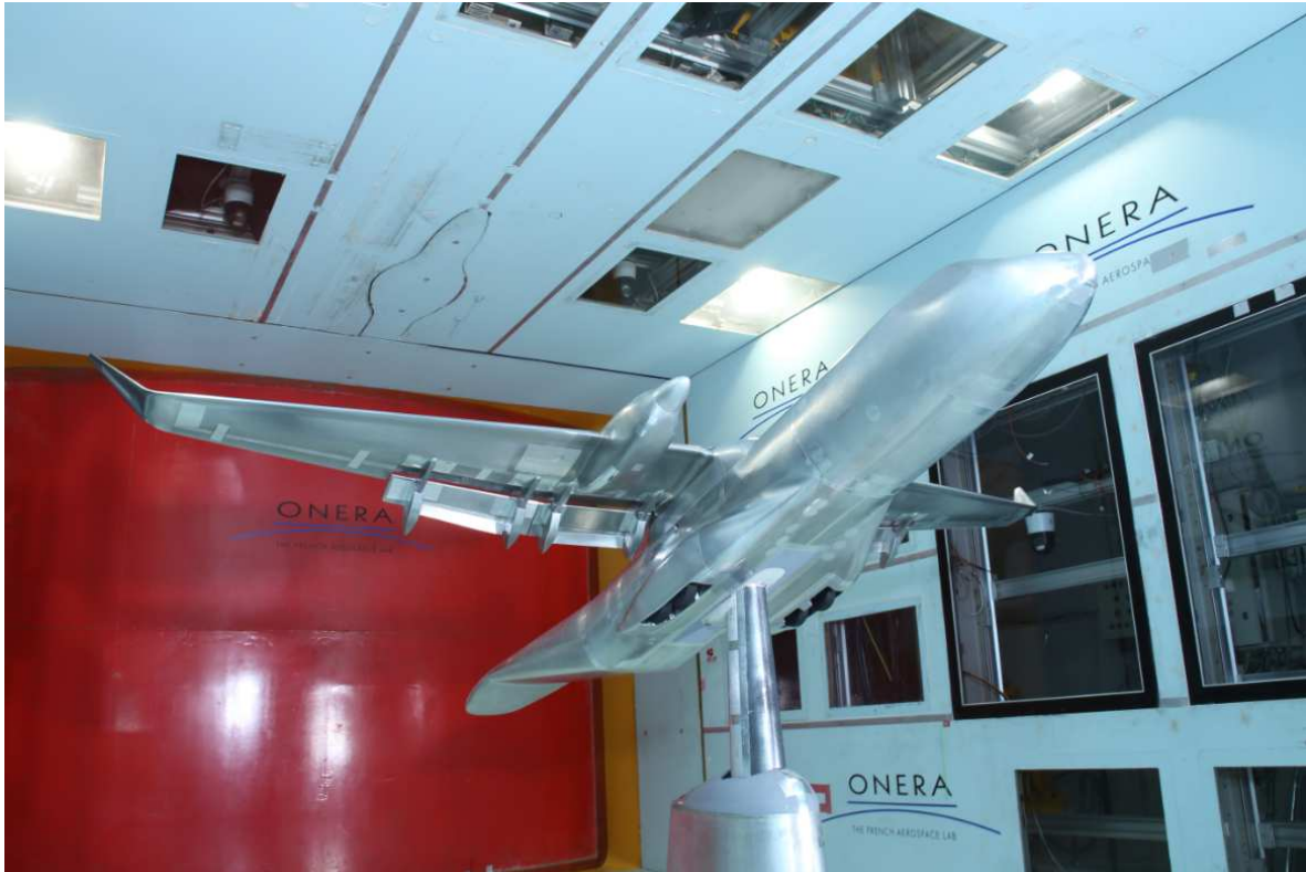
Figure 8 –Model in ONERA F1.
