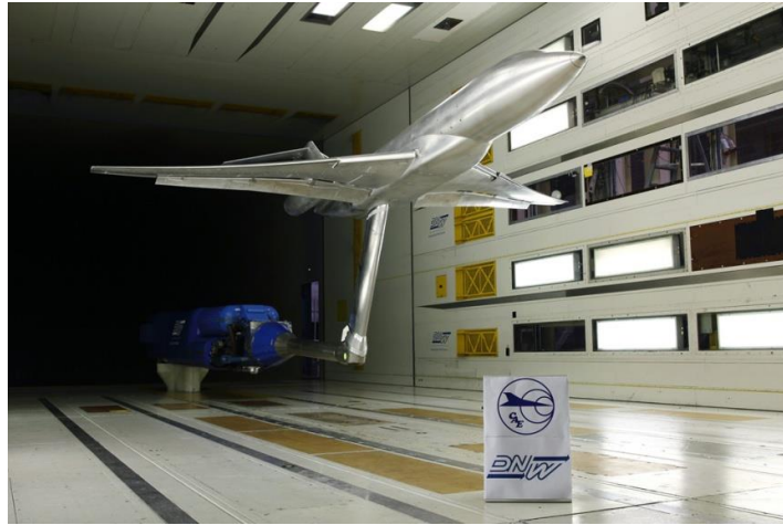
Figure 11 – CAE-AVM-HL model tested in DNW-LLF 8x6 meter test section
