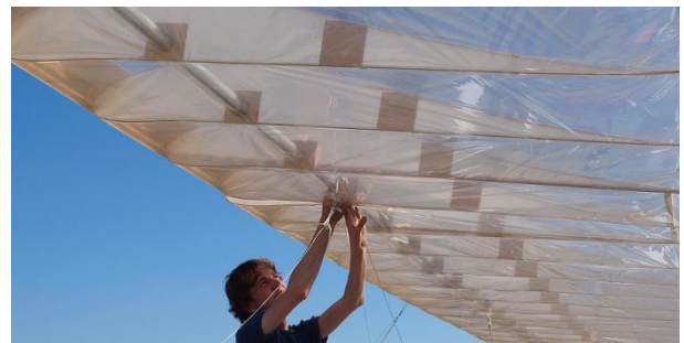
Fig. 4. Detail of the wing, showing wing ribs, main spar, Mylar skin and the author.
