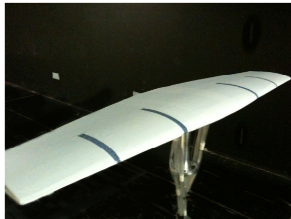
Figure 2: Manufactured NACA 2313 wing featuring pressure insert modules at 4 span wise locations.
