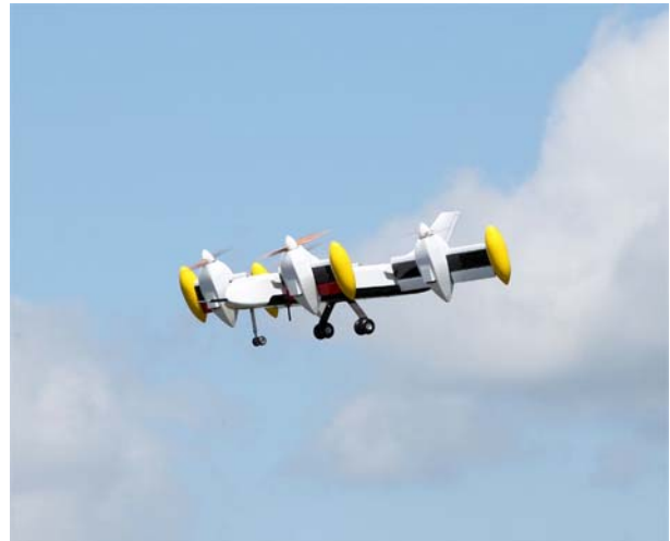
Fig. 12 The Next Prototype (Mission capability technology demonstrator, Gross Weight = 43kg, Span=2.4m)
