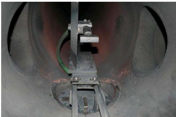
Fig. 9 The cylindrical instrumented model in the X2 test section during the test campaign
