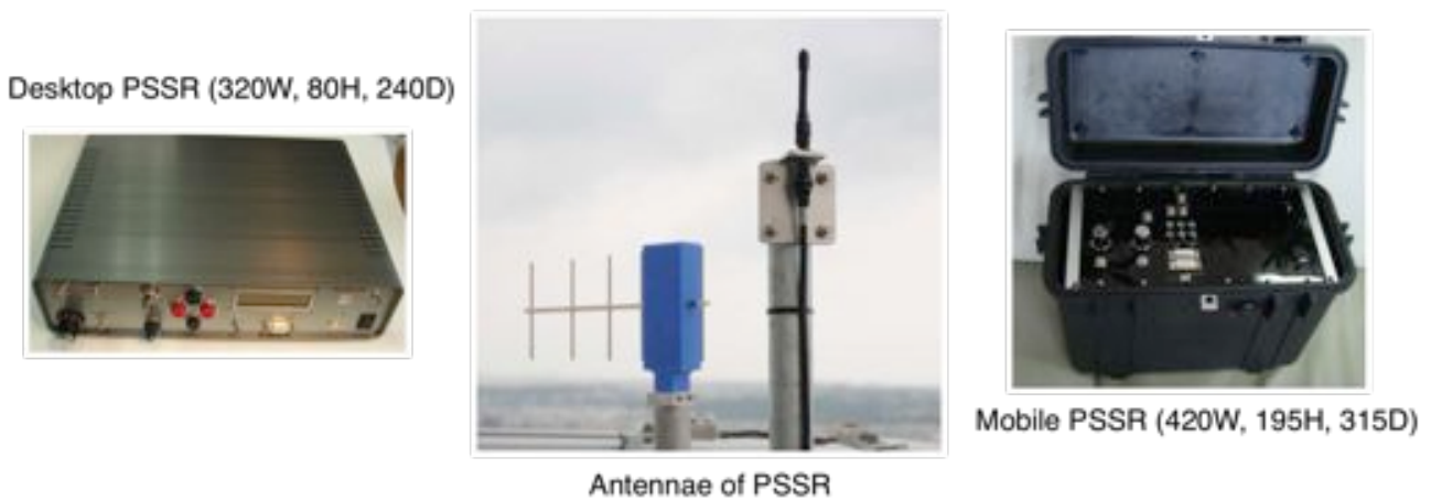
Fig. 7 Latest PSSR Signal Processors (Desktop PSSR S.P. & Mobile PSSR S.P.) and the Antennae (Yagi Antenna & Omnidirectional Antenna)
