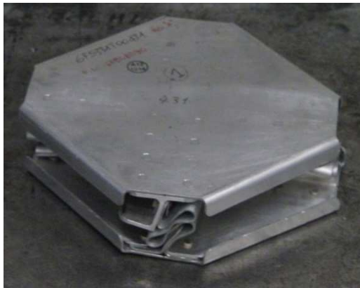
Fig. 2 - Intersection cruciform element after test
