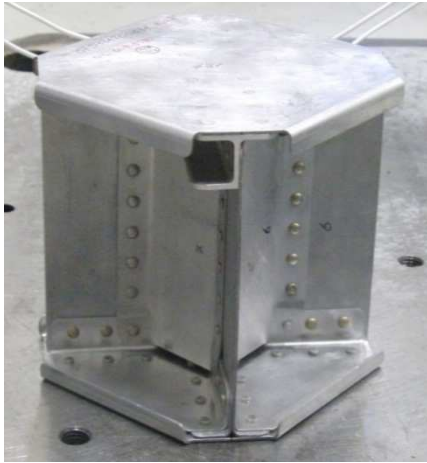
Fig. 1 - Intersection cruciform element before test
