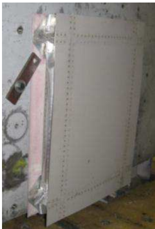
Fig. 5- Subfloor cell after test
