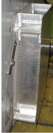
Fig. 4- Subfloor cell before test
