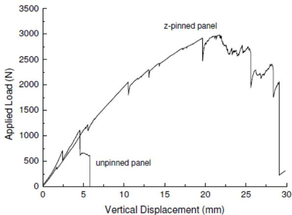
Fig. 7. Applied load-displacement curves for the T-joints with and without z-pins containing a pre-existing 20 mm long delamination crack. The z-pinned joint had a pin content of 2% by volume.
