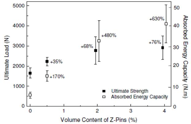
Fig. 6. Effect of volume content of z-pins on the ultimate strength and absorbed energy capacity of the defect-free T-joint. The percentage increase to the property values due to z-pinning are given.
