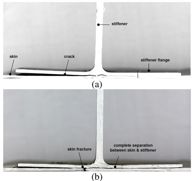
Fig. 11. Unpinned T-joint specimens following impact loading at energy levels of (a) 8 J and (b) 14 J.
