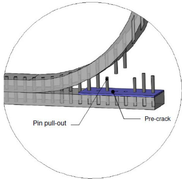
Fig. 9. Schematic of the crack opening displacement and z-pin bridging traction zone in a T-joint containing a pre-existing crack. The length of the bridging traction zone was not dependent on the initial pre-crack length.
