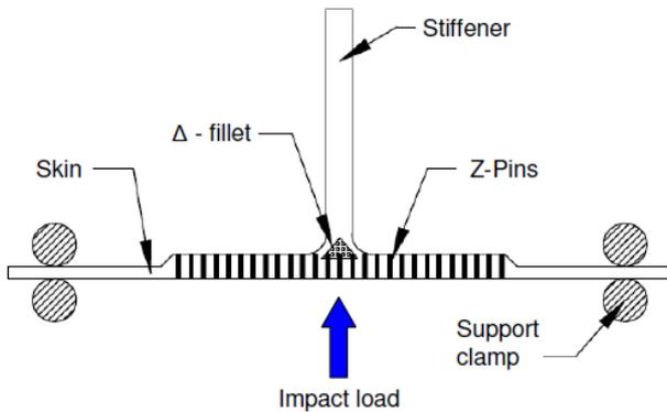
Fig.3. Schematic of T-joint specimen reinforced with z-pins subjected to impact loading.
