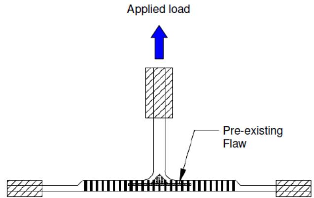
Fig. 2. Schematic of T-joint specimen reinforced with z-pins containing a single bond-line crack.
