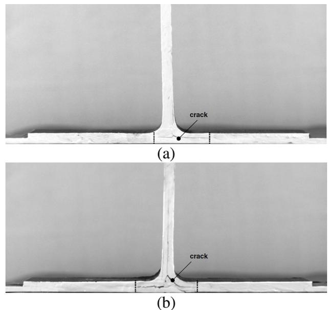
Fig. 12. Z-pinned T-joint specimens following impact loading at energy levels of (a) 8 J and (b) 14 J.
