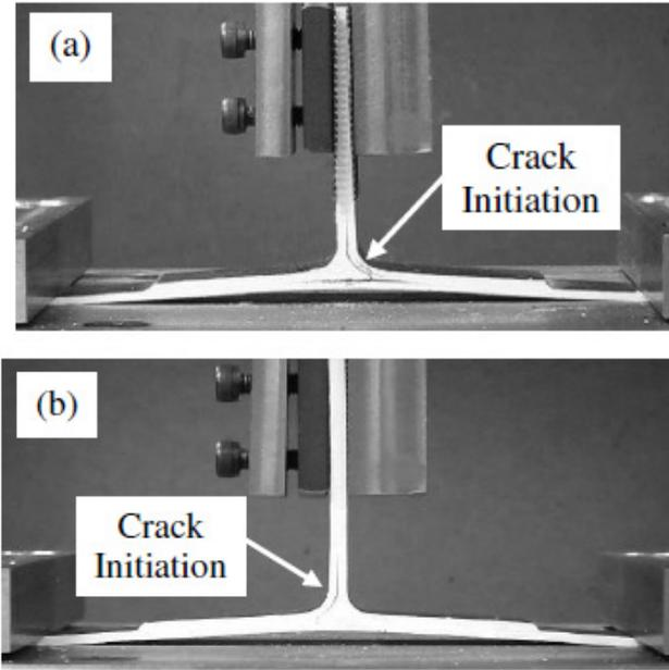
Fig. 5. Damage in the defect-free T-joints (a) without z-pins and (b) with z-pins when loaded to the failure initiation stress. The z-pinned joint had a pin content of 2% by volume.
