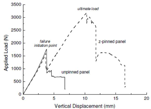
Fig. 4. Applied load-displacement curves for the defect-free T-joint with and without z-pins. The z-pinned joint had a pin content of 2% by volume.
