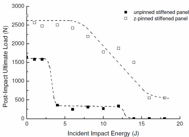
Fig. 13. Effect of incident impact energy on the post-impact ultimate load of the unpinned and z-pinned joints. The z-pinned joint had a pin content of 2% by volume.
