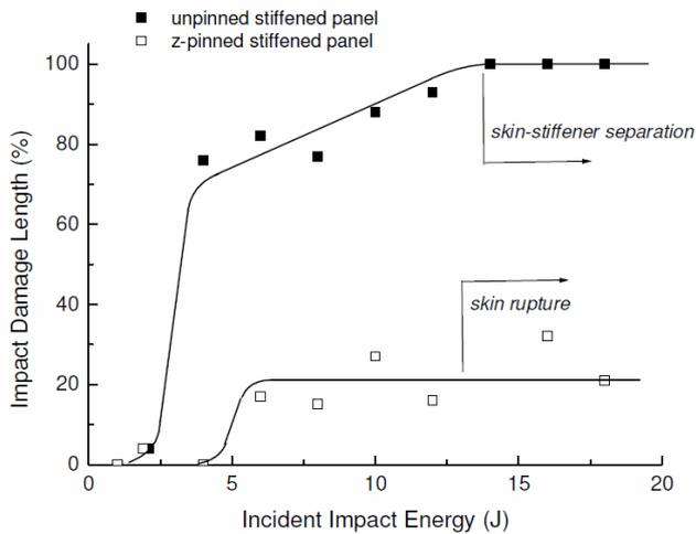
Fig. 10. Effect of incident impact energy on the delamination crack length in the unpinned and z-pinned T-joint. The delamination length is expressed as a percentage of the total bonded length (100 mm). The z-pinned joint had a pin content of 2% by volume.
