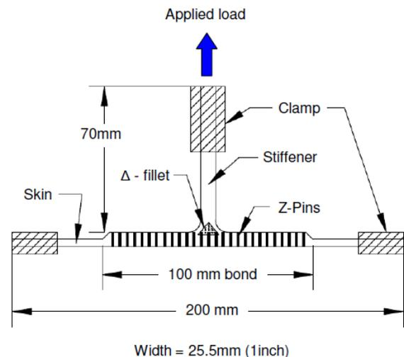
Fig. 1. Schematic of T-joint specimen reinforced with z-pins. The dimensions, boundary (clamping) conditions, and load direction are indicated.
