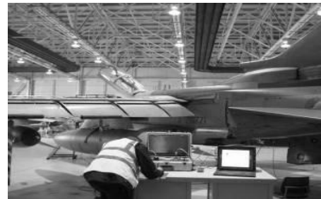
Fig 5. IFD Testing of Tornado CDC
