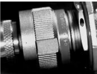
Fig 9. Mission System Cable Connector; Fully Locked
