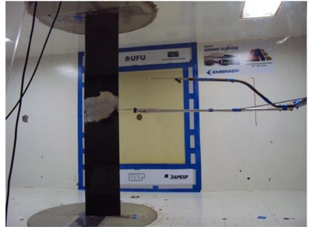
Fig. 8. Experimental set-up for boundary layer measurements with hot wire.
