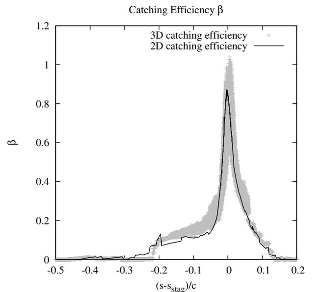
Fig. 5 : Three dimensional catching efficiency for NACA 23012 at an MVD of 236  $\mu\text{m}$
