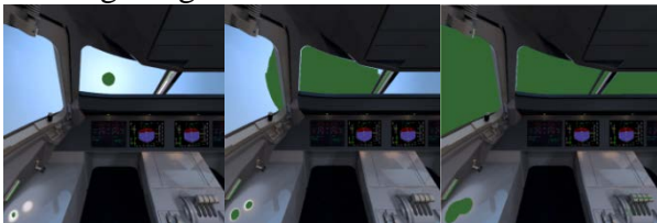
Fig.5. Glare detected result of the flight deck.
