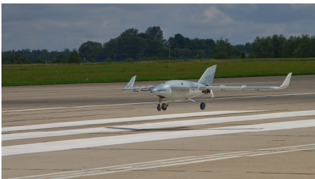
Fig. 8 Tailless, pushing propeller airplane after flight show, just before touchdown. Minsk Mazowiecki, July 2011.
