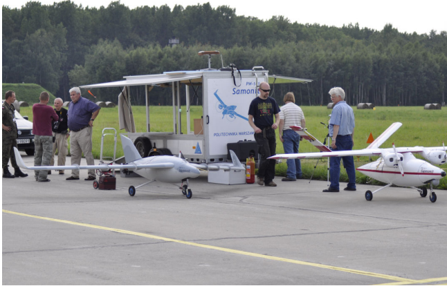
Fig. 7 Ground preparation for flight-testing. Tailless, pushing propeller airplane on the left, the classical V-tail configuration on the right and Ground Control Station (also used for transport of airplane parts) behind. Minsk Mazowiecki, July 2011.
