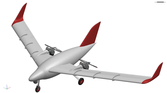
Fig. 4 SAMONIT in tailless configuration with pushing propellers
