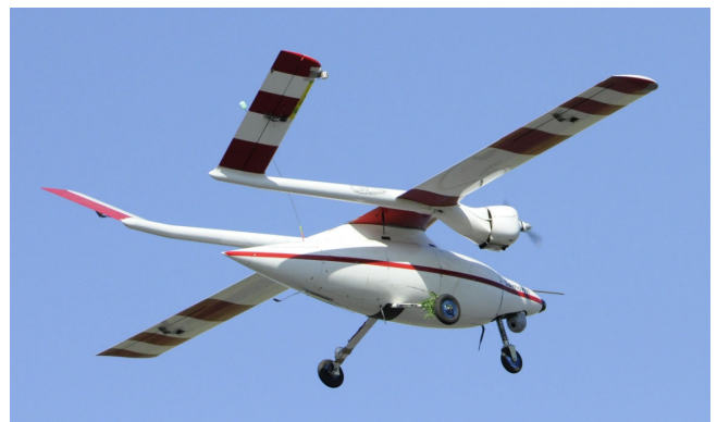
Fig. 5 Airplane in tailed, tractor configuration. Flight test with autopilot in the loop. Daylight camera (FLIR) visible at the nose of the container. Sochaczew, April 2011.
