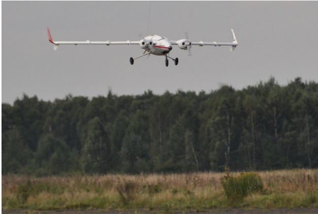
Fig. 6 Airplane in tailless, tractor configuration. Flight test in manual mode. Daylight camera visible at the nose of the container. Sochaczew, September 2010.
