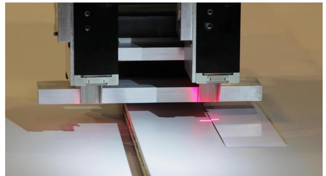
**Fig. 3** Photograph of the setup with edge detectors (1), material edge (2) and laser light section (3)
