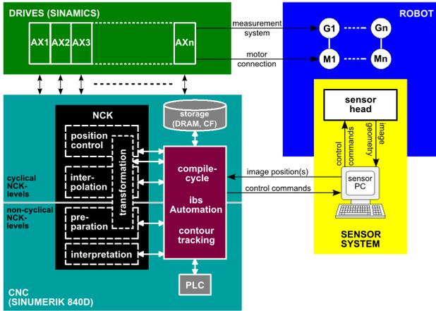
**Fig. 5** Data flow of the CNC-integrated contour tracking
