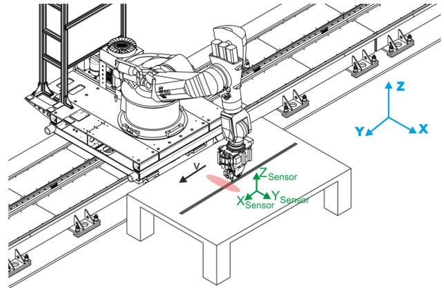
**Fig. 2** Test setup with illustrated coordinate systems) - blue: global coordinate system, green: sensor coordinate system
