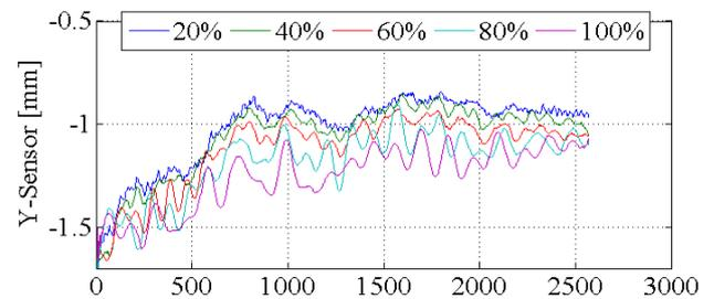
Fig. 10 Linear axis motion with all speeds - 20%=6m/min, 40%=12m/min, 60%=18m/min, 80%=24m/min, 100%=30m/min
