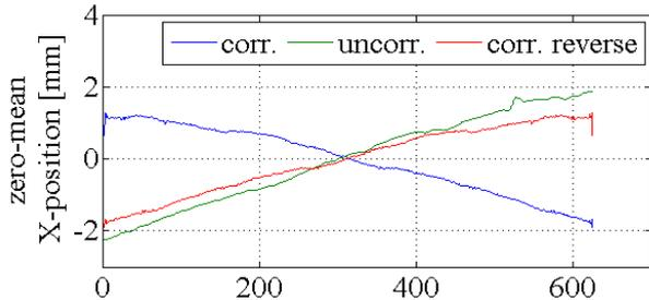
**Fig. 14** Comparison of a corrected with an uncorrected edge detection
