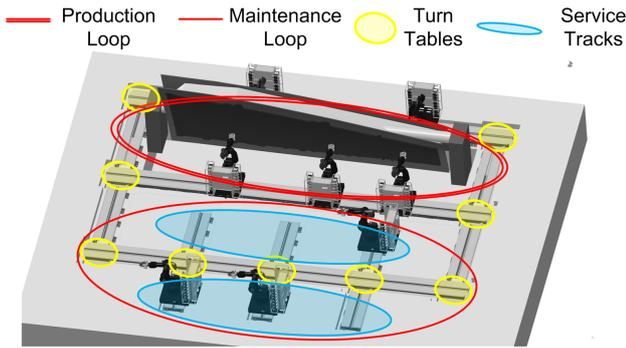
**Fig. 1** Automated Fiber Placement facility with 8 coordinated robots laying up on a double-sided molding tool
