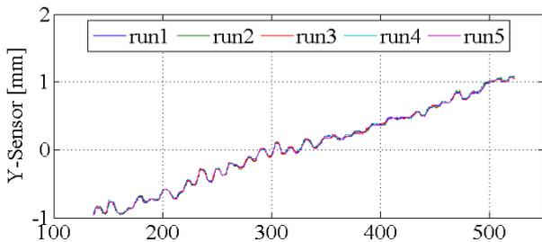
Fig. 9 Measurement series of the Y-position with 30m/min and combined linear and robot motion
