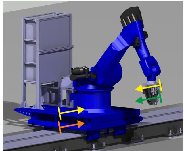
**Fig. 4** Representation of the different motion characteristics - orange: moving platform, green: moving via robot axes, yellow: combined moving platform and robot axes
