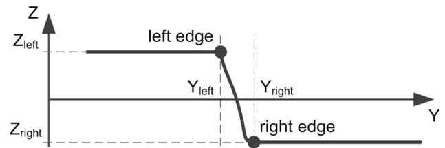
**Fig. 6** Scheme of the co-ordinate system of the laser stripe sensor
