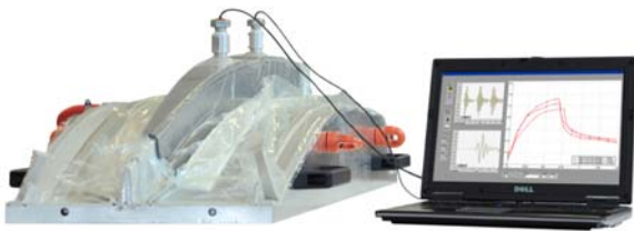
Fig. 2. Cure Monitoring by Ultrasound
