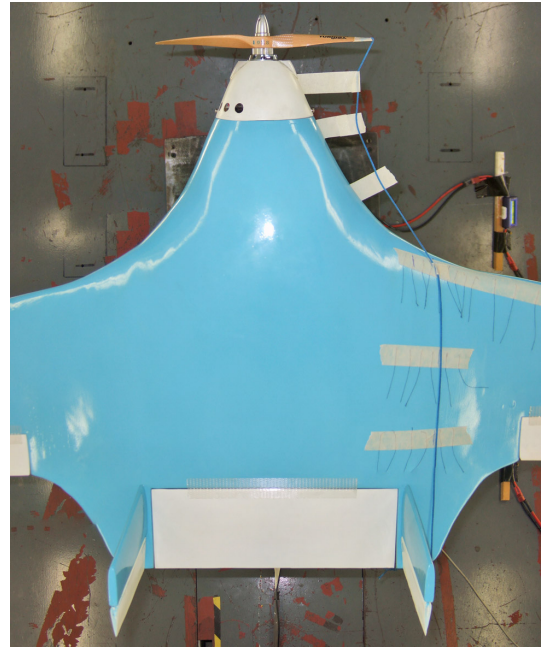
Fig. 14 Prop wash boundary as determined in the wind tunnel for a 10 inch propeller
