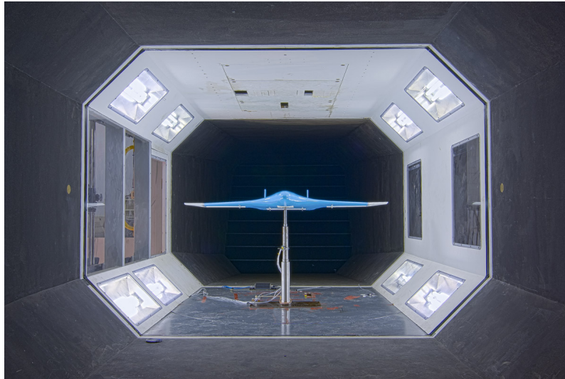
Fig. 3 Wind tunnel installation with fairings removed
