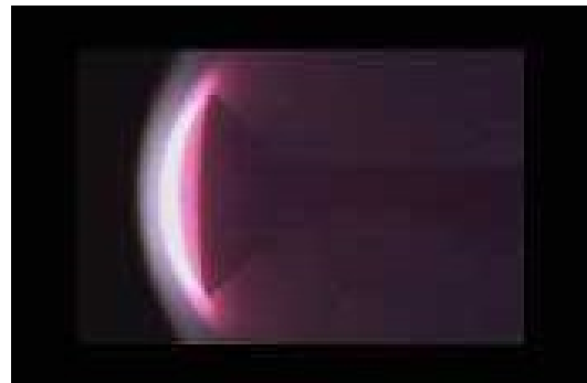
Fig. 4 Image of bow shock in expansion tube test
