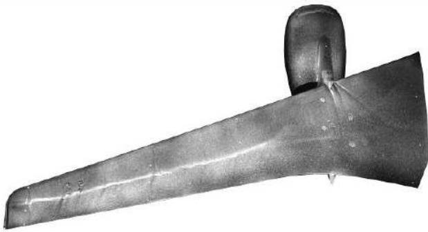
Fig. 4. Model after wind tunnel test with the oil viscosity of 60000 cSt.
