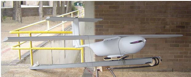
Fig. 11. The SUAVE UAV on its launcher.
