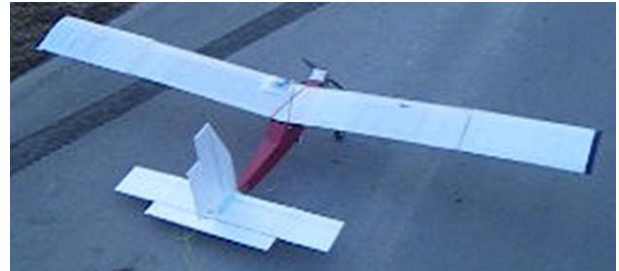
Fig. 17. Spring Hinge Type Folding Method Airplane.
