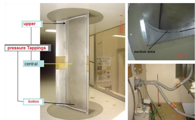
Fig. 4 High lift experimental set-up with wind tunnel wall boundary layer suction.
