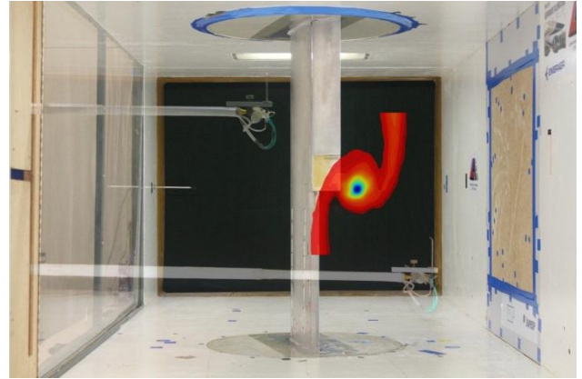
Fig. 25 Vortex and wake mapping , \alpha=12^\circ .
