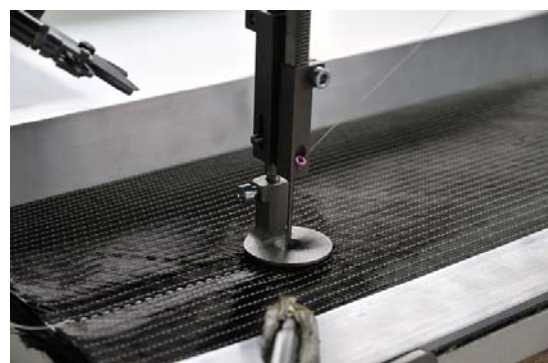
Fig. 7. Tufting of a specimen with doubler face down
