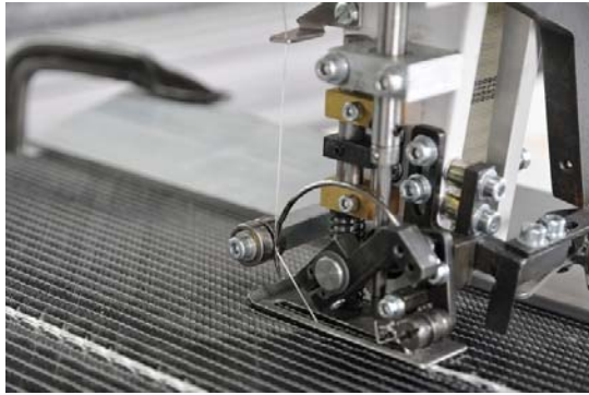
Fig. 8. Blind stitching of a specimen – notice curved needle
