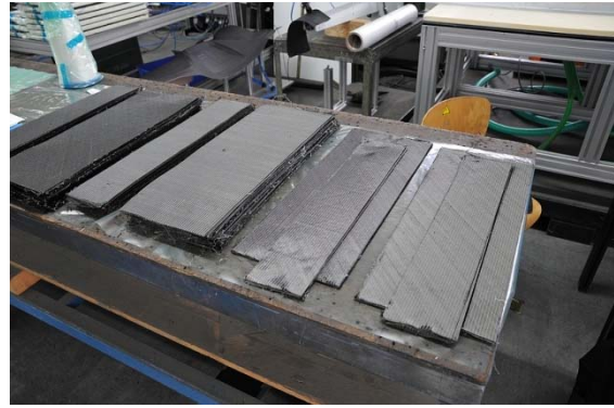
Fig. 6. Cut NCFs in waiting of layup
