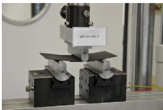
Fig. 9. Skin-doubler 3 point bending specimen in test rig [6]
