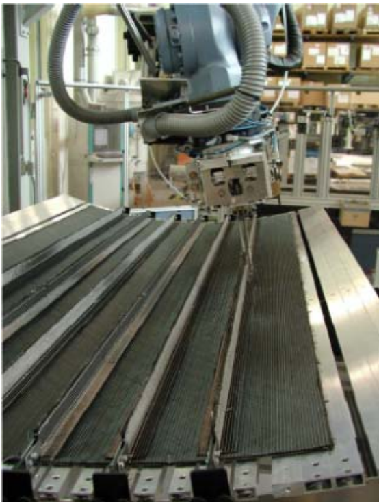
Fig. 2. Selective stitching of stringers on curved panel, from Baisch [2]
