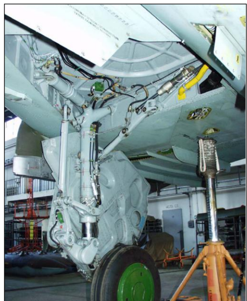
Fig. 10. View of the main landing gear
