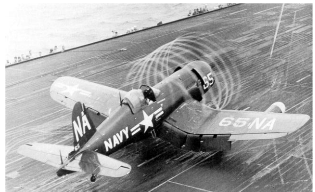
Figure 3. Propeller slipstream condensation of Vought-F4U-Corsair [11].
