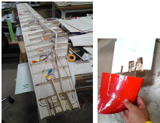
Fig.5 Wing Structure and Wing Tip Separation Mechanism
