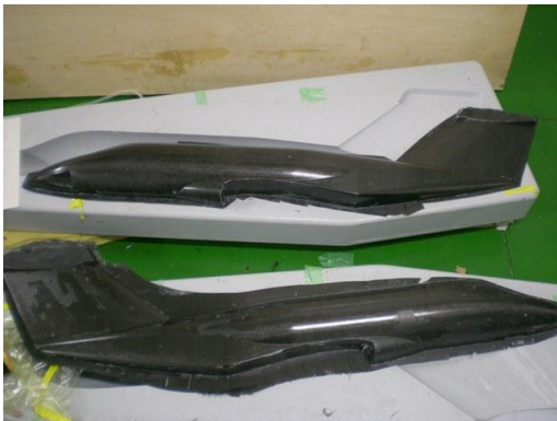
Fig.4 Fuselage and Vertical Tail made of CFRP
