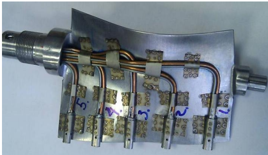
Fig. 1.3. S1 blade, instrumented by deflectors with total pressure tubes and thermocouples
