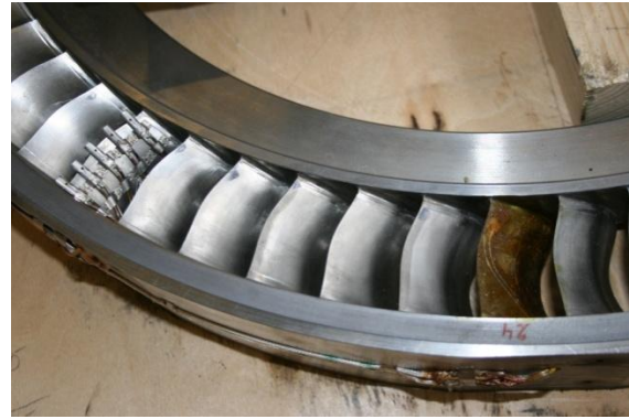
Fig. 1.5. S2 stator blades – monoblock, instrumented by strain gauges and total pressure and temperature sensors
