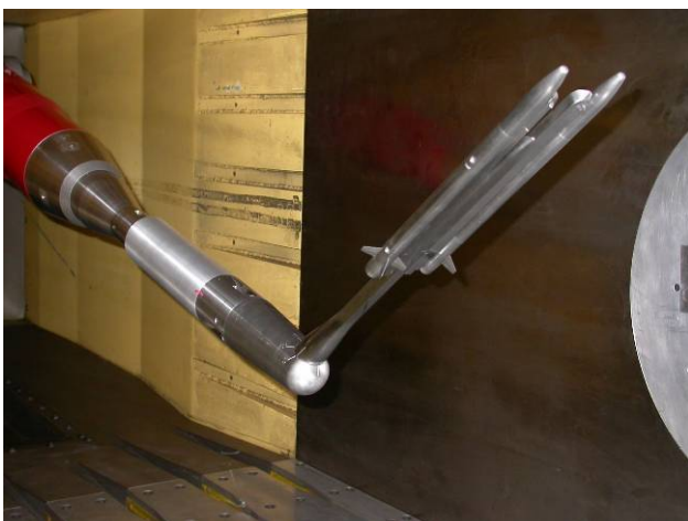
Fig. 7 Dual AIM-120 and LAU-127 launcher mounting system in the DSTO Transonic Wind Tunnel
