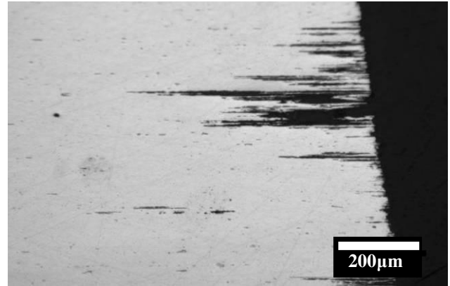
Fig. 8. Example of IGC using 3.5% NaCl, 1.2% H_2O_2 solution exposed for two weeks.
