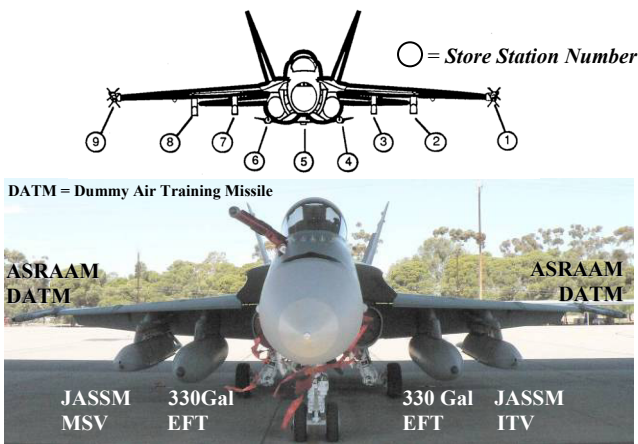
Fig. 4 GVT and Clearance Station Configuration
