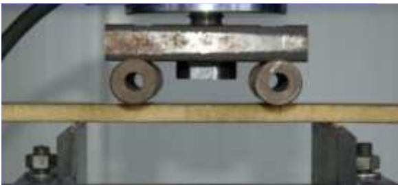
Fig. 5. Sandwich specimen bending test
