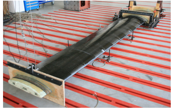
Fig. 14. Static test of compact wound segment
