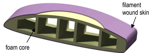
Fig. 1. Schematic visualization of investigated sailplane wing structure
