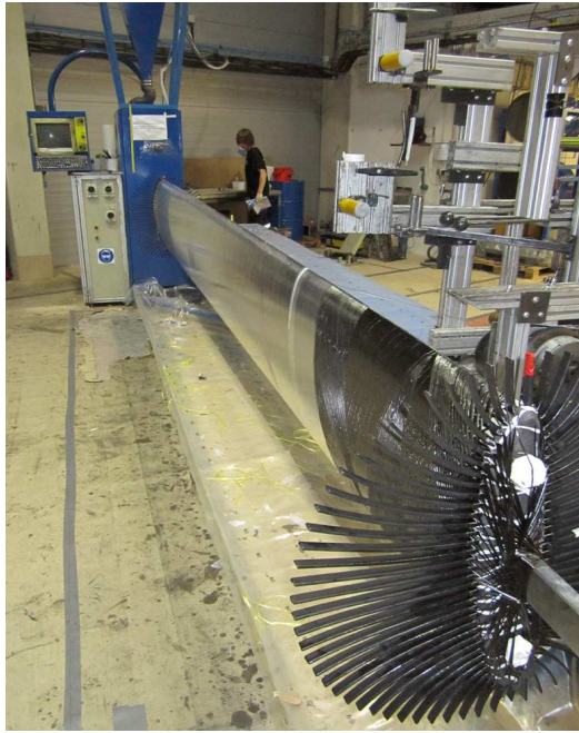
Fig. 13. Wing segment during winding
