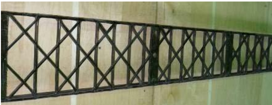
Fig. 7. External and internal views of a composite geodesic fuselage section
