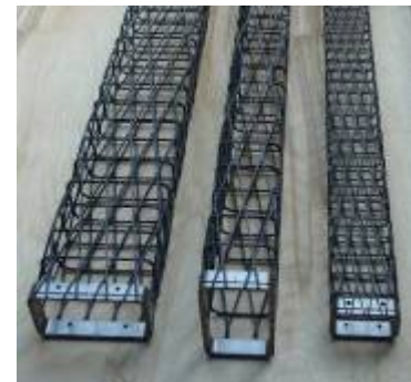
Fig. 7. External and internal views of a composite geodesic fuselage section
