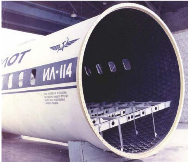
Fig. 7. External and internal views of a composite geodesic fuselage section
