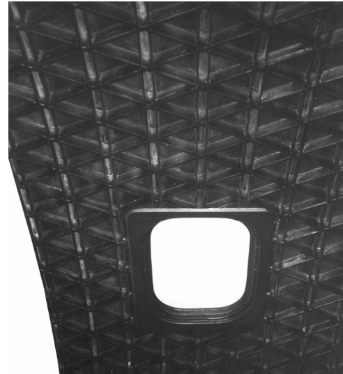
Fig. 7. External and internal views of a composite geodesic fuselage section
