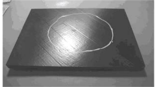
Fig. 3. Delamination area in quasi-isotropic 8 mm thick carbon-epoxy laminate after impact with energy 35 J
