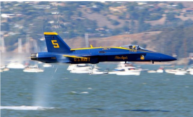
Fig. 1. A US Navy Blue Angels demonstration aircraft at approximately Mach 0.95 (photo: Matt Niesen).
