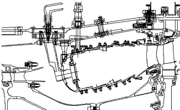
Figure 4. Trent ‘Phase 5’ tiled combustor and combustor design space & requirements
