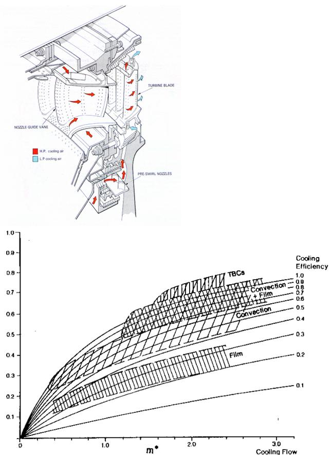
Figure 12: a) typical HPT cooling arrangement and b) Cooling effectiveness of different cooling types.
