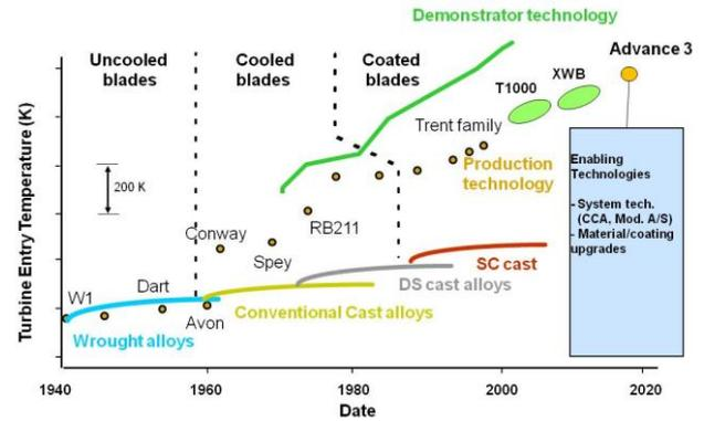
Figure 11: Development of HPT blade system Turbine inlet temperature capability
