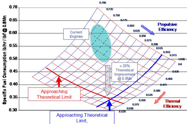
Figure 2: SFC as a function of propulsive and thermal efficiency
