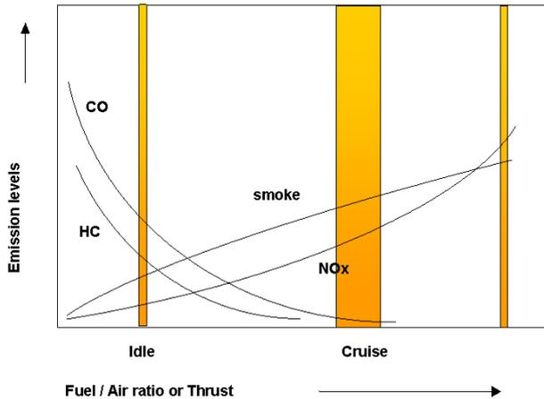
Figure 8: Aero-engine emissions characteristics
