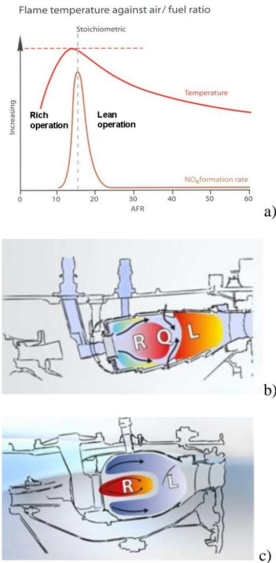
Figure 10: NO<sub>x</sub> formation (a), Rich (RQL) (b) and lean combustion topology (c)
