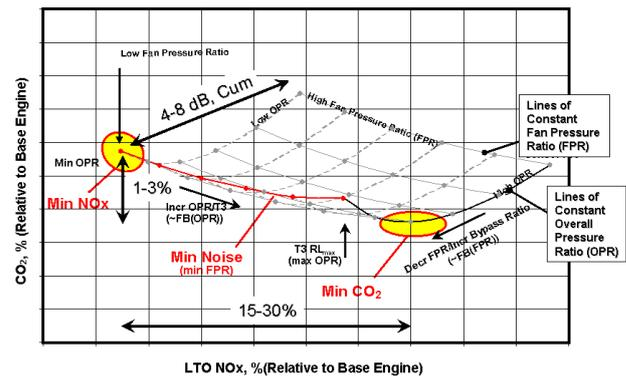
Figure 9: Aero-engine Optimisation trades for new engine design [4]
