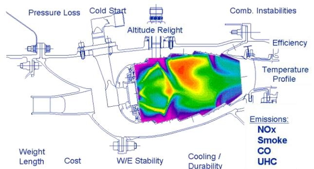
Figure 7: Design requirements for the overall combustion sub-system [4]
