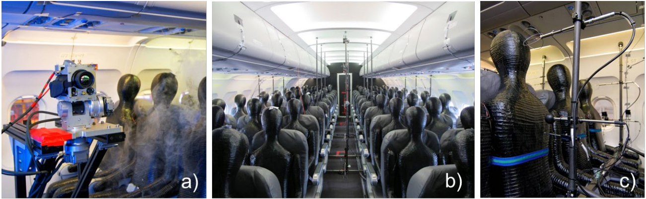
Fig. 3. Photographs of the flight-test installation in the measurement section. a) Automatically rotateable infrared camera set-up for acquisition of surface temperature panoramas during the flight, b) thermal passenger dummies, sensor racks and surface temperature sensors, c) thermal passenger dummies and SR1 sensor rack.
