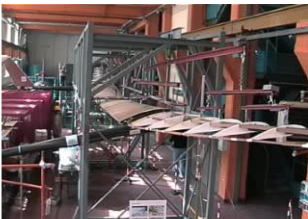
Fig. 8 - 1:3 Scaled-size HeliPlat® UAV – Shear/Bending and Torsion Tests
