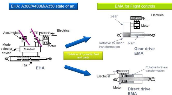
For Sagem, in order to choose adequate technologies regarding optimized wings surfaces control, we have taken the major hypothesis that all technologies will cooperate, EHA and EMA, for front line as for back-up actuation systems. Moreover some type of aircraft will still retains HA solution as the most suitable technology.
