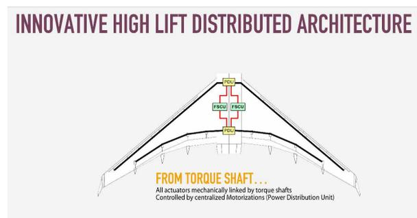
The figure above shows current High Lift system architecture on any aircraft.
