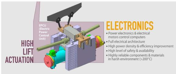
About electrical motors topology, very stringent safety and reliability requirements are permitted, thanks to the electrification, optimizing at the same time system mass and volume, and easiness in installing and maintaining it at aircraft level.
