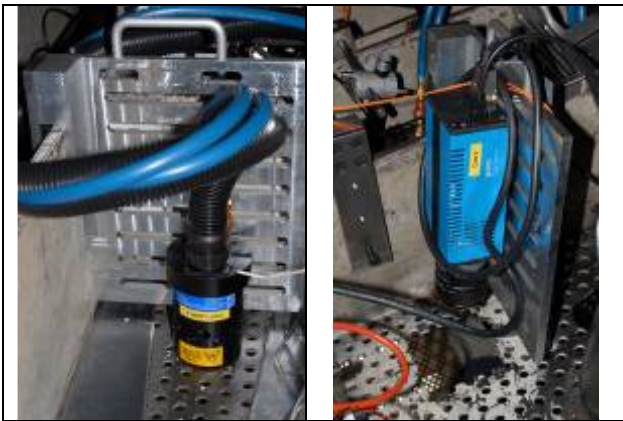
Fig 5 TSP camera and lamp installation with the TWT plenum roof area.
