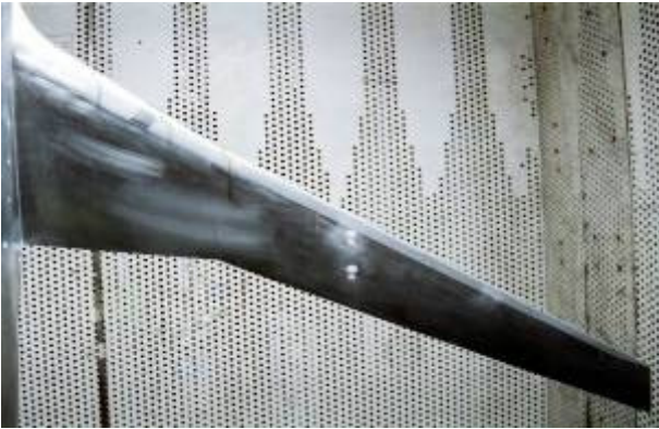
Fig 8 Sublimation photograph showing result of transition fixed at 0.15c.
